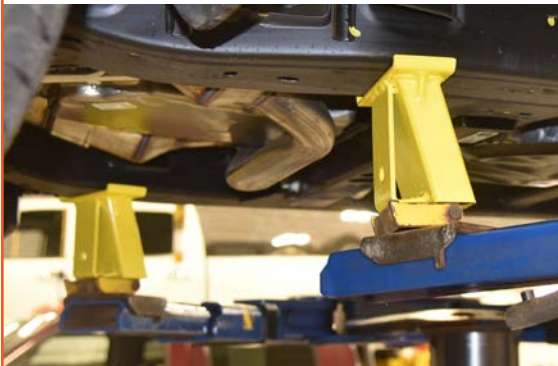
Front Adapters have 7" Wide Lifting Area
