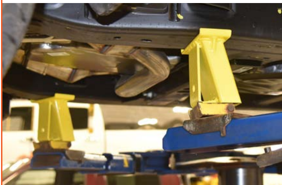
Front Adapters have 7" Wide Lifting Area
