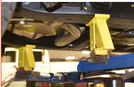
Front Adapters have 7" Wide Lifting Area
