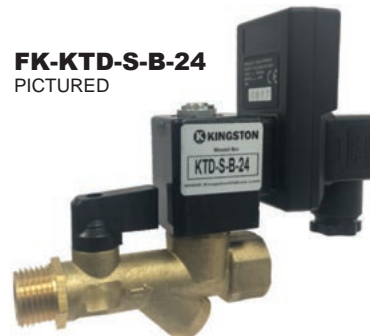
Electronic Timer Drain with Ball Valve and Strainer 1/2" Male & 1/4" Female NPT inlet x 1/2" Female NPT outlet, 110 VAC, 60 Hz SVI Part #: FK-KTD-S-B-24
