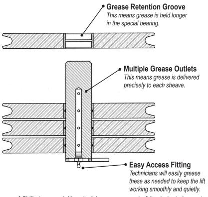
Solving the needs of all lift industry distributors remains one of SVI's top specialties. In this case, several of the industry's most respected distributors asked us to develop greaseable sheaves and sheave pins for 4-post lifts to reduce the frequency with which standard sheaves and pins are replaced.
