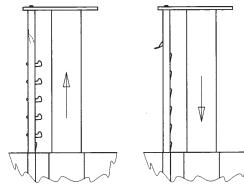
When it is time to lower the lift, simply pull down on the handle to disengage all the locks.
