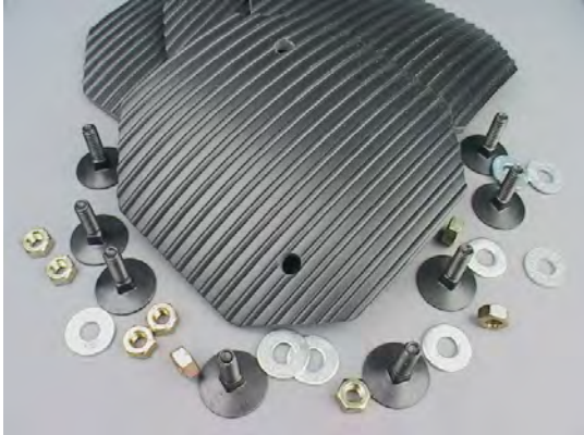
Rubber Arm Pad Kit for Forward Lifts BH-7235-90 (Ref 994105)
