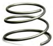
RM-45500 (Ref 90630, 903590, 3590, 45500) Spring for Centering Cone This tapered spring works same as straight spring. The taper allows the spring to fold in on itself as it is compressed, giving a little extra room to allow the cone to center in the rotors/drums.
