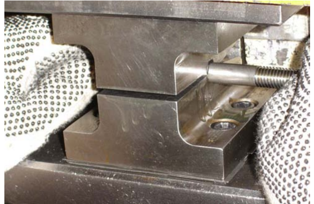
Cable end being swaged on 5/16" wire rope
