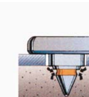
Set When fully driven, the displaced metal is permanently embedded in the locking groove.
